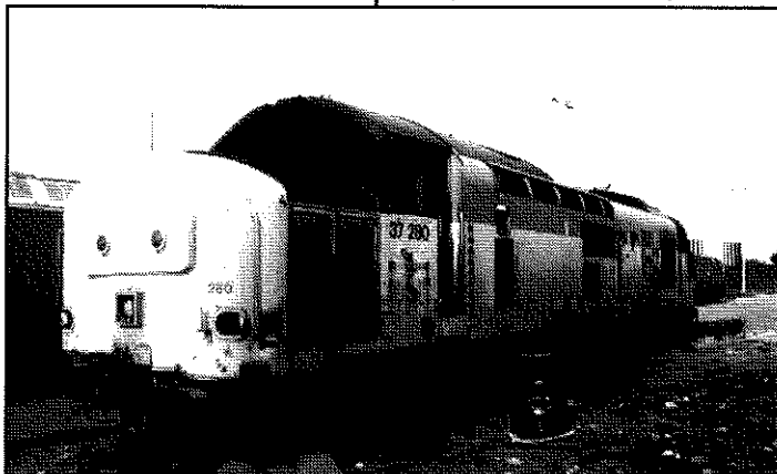
Withdrawn 37280 has been heavily robbed of parts as it sits without bogies at Old Oak Common depot. This is just one of the locos featured in our location round-up listed left. Photo: D. JENNINGS
