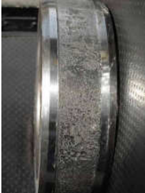
Bit tired! The old inner bearing race.
