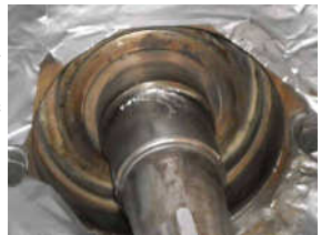
All gone: the shaft with the old bearing fully off.
