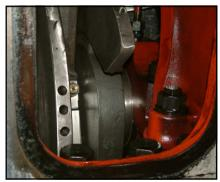
In a standard Class 37 engine bay, you can barely squeeze past the power unit. 37905's 6 cylinder, in-line RK270 experimental power unit affords the fitter enough room to swing a cat. Phil Lynch was clearly very tired when this picture was taken.
