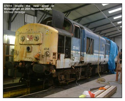
Some time has also been spent on the loco too though. Mick Chester and Phil Broadbent spent a few weekends stripping the top end of the power unit and disconnecting it ready for removal at a later date. It is now very likely that we will be fitting a fresh power unit in '414 rather than rebuilding the one we have. Phil and the bodywork team have also started to prepare the loco for repainting.
