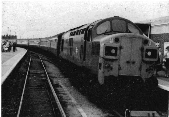
37107 has arrived at Yarmouth with the 1015 from Birmingham New Street on 6.8.83. Many of the original features are retained, including skirts and glass headcode panels. It is xb, March allocated.
